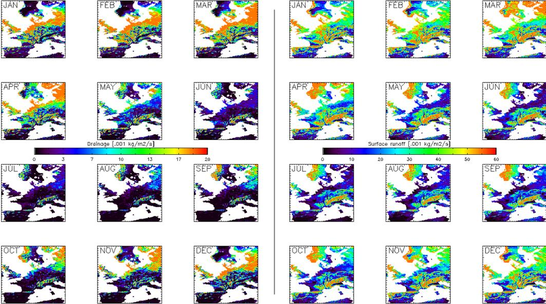
Figure 5: Monthly mean climatology for drainage (left) and surface runoff (right).
